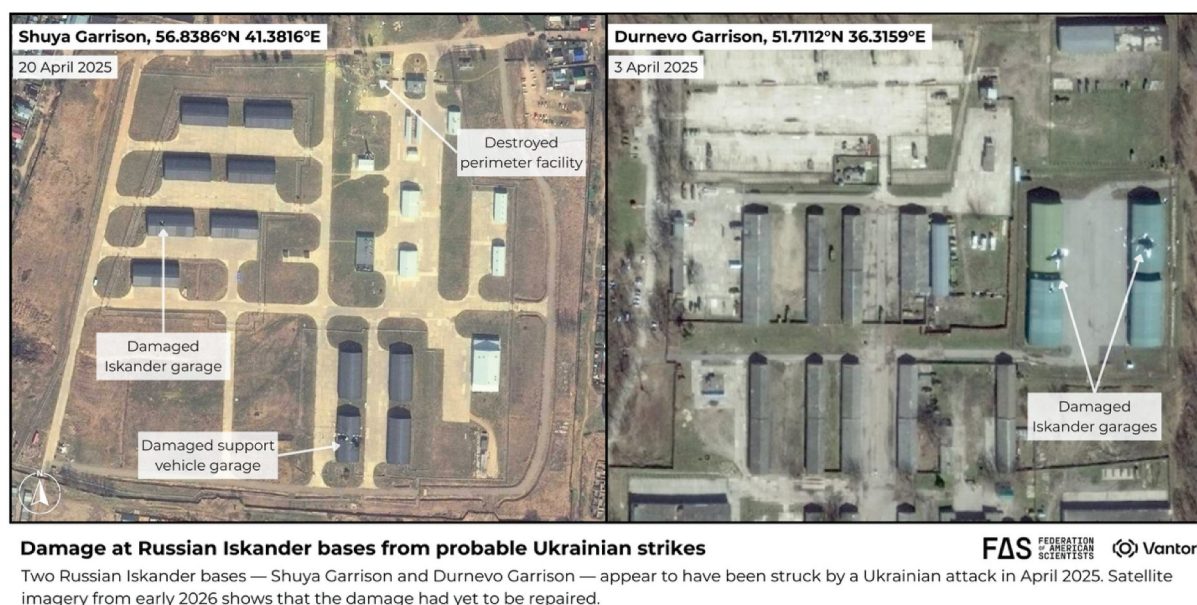
Figure 5. Damage at Russian Iskander bases from probable Ukrainian drone strikes (Credit: Vantor/Federation of American Scientists).
